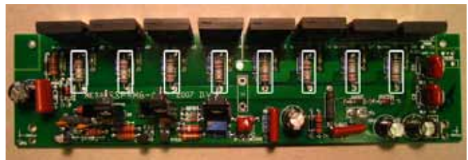
Fuse-type Source Resistor location on Carbine
