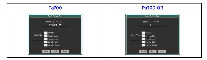
19) *Dial/Value Test:* Rotate the DIAL clockwise, until you read +48; then rotate it counterclockwise, until you read -48; at this point, the check box should become green.
