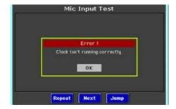
In this case turn the instrument off, insert the battery (if it isn't already inside the battery socket) and turn the instrument on again. Wait for the default screen, then set the date and time:
